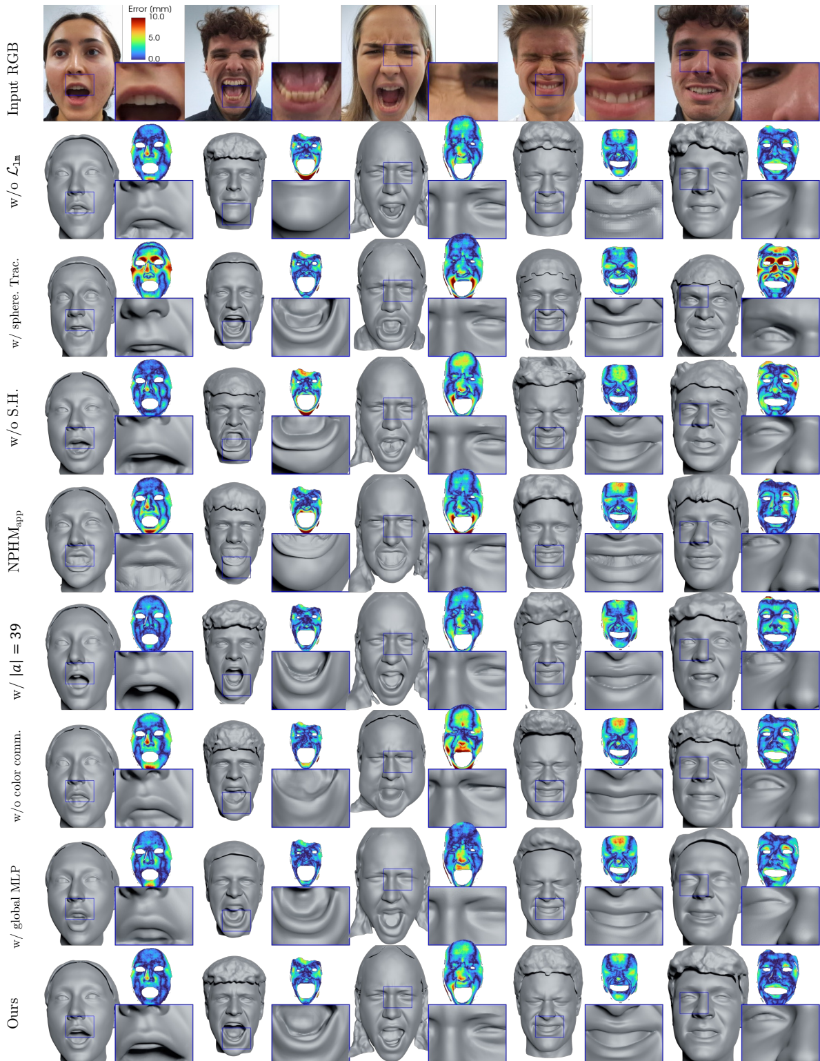
Figure 3. Ablation Results: Qualitative comparison of our ablation experiments, as quantitatively reported in Table 2 in the main document. Rows and columns are transposed compared to our other result figures. The error maps show the color-coded point-to-mesh distance from the back-projected Kinect depth to the reconstruction. See Sec. 3.2 for a description of our findings.
