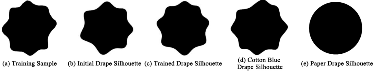
Figure 11. Through digitalization ( i.e. training BDP), cloth drape silhouette (b and c) is optimized toward the training sample(a). In addition, (d) shows the simulated Cusick drape silhouette of a paper-like material.
