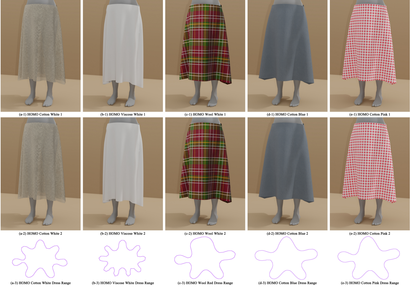
Figure 9. The clothes digitalized by the HOMO model is deterministic and has homogeneous material properties. Thus, the simulated dresses that are made from the same cloth always have the identical geometry.
