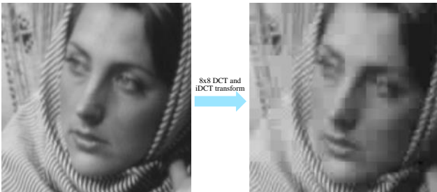
Figure S1. 8 \times 8 block-wise DCT and iDCT transform leads to severe visual discontinuity. Zoom in for more details.
