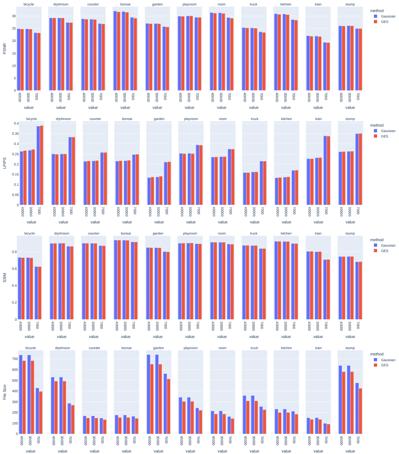
Figure 33. Detailed Per Scene Results On MipNeRF 360 for Different Iteration Numbers. We show PSNR, LPIPS, SSIM, and file size results for every single scene in MIPNeRF 360 dataset [5] of our GES and re-running the Gaussian Splatting [27] baseline with the exact same hyperparameters of our GES and on different number of iterations.
