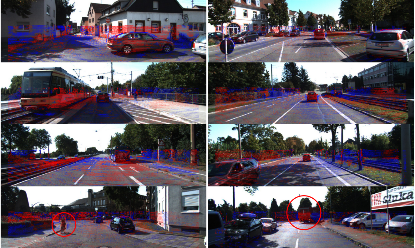
Figure 15. Depth error comparison between BTS and KDBTS. KDBTS exhibits slightly more large errors compared to BTS. Qualitative examples (bottom) demonstrate depth error on the KITTI test set, with lower errors depicted by KDBTS (blue dots) and BTS (red dots), with intensity representing magnitude. Each test image presents the projected scene from the LiDAR ground truth point cloud. The projected LiDAR point cloud is used to calculate the distance error between the prediction and its ground truth. Color differentiation indicates lesser distance errors between KDBTS (blue dots) and BTS (red dots). In KDBTS, the model's reconstruction is affected by moving objects, resulting in larger errors typically observed on dynamic objects (e.g., cars, cyclists). Consequently, red dots are depicted for dynamic objects, signifying lower errors for BTS.
