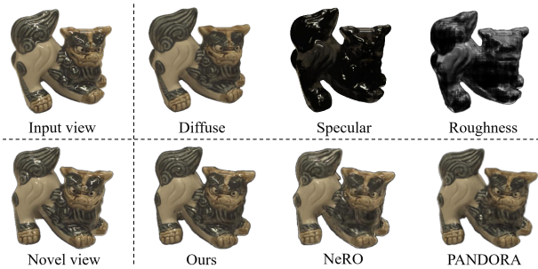
Figure S4. (Top) Estimated BRDF from our method. (Bottom) Comparison of novel view synthesis.
