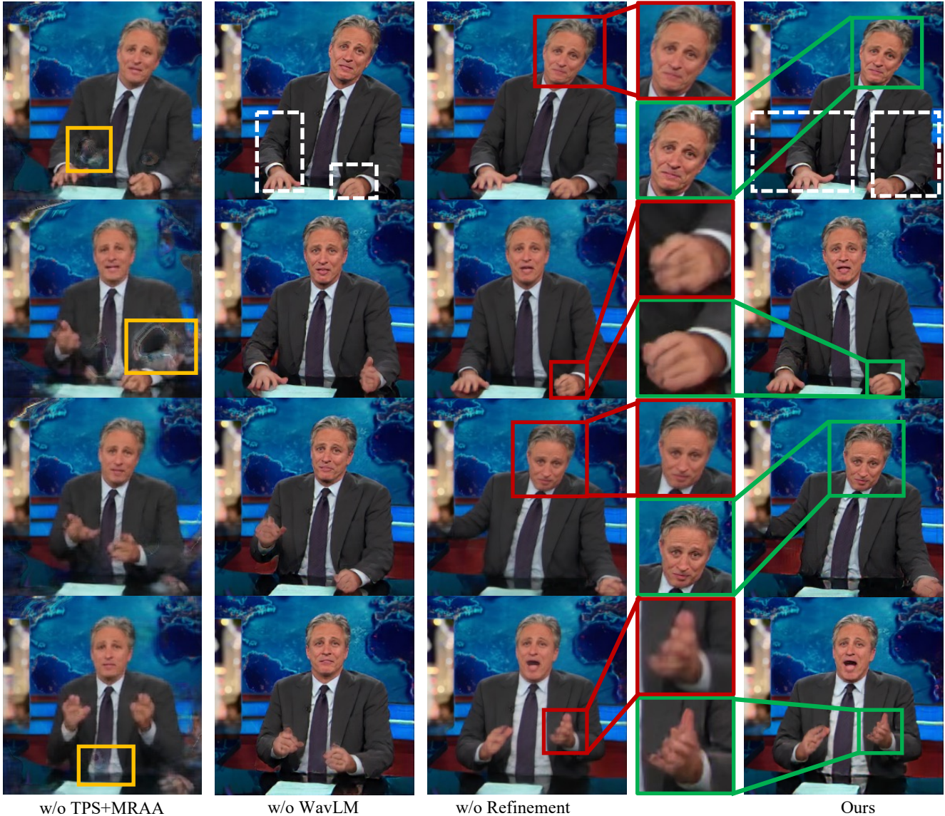
Figure E1. Visualization results of the ablation study. Replacing TPS with MRAA leads to ghost effects (yellow boxes). WavLM brings greater amplitude of hand motion (dashed boxes) given an impassioned speech. Refinement restores the details especially in hands and the face (red and green boxes).
