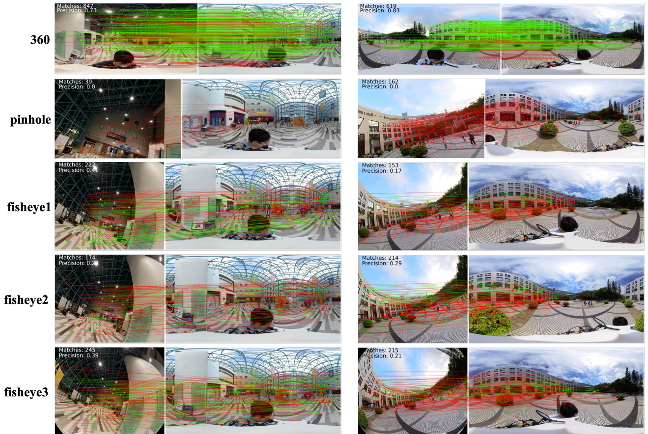
Figure 4. Two groups of local 2D-2D matching pairs (Superpoint + LightGlue [7]). For each pair, left side is the query frame and right side is the top-1 retrieved reference 360° image. In this figure, all retrieved images are correct. The reprojection error threshold is 5px (green means correct matches, red means wrong matches).
