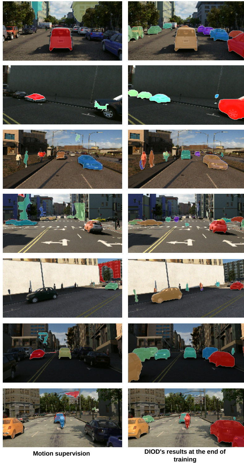
Figure 6. Illustration of the improvement achieved by DIOD as shown in column 2, leveraging the noisy and sparse motion masks (column 1) to direct the slots' attention. These example frames are from the training set of TRI-PD [2]
