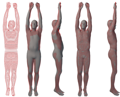
Figure 8. Examples of the obtained fit results. Left: point-cloud S_i extracted from the MRI. Middle: Volume preserving SMPL model fit S_i . Right: Free-vertex fit F_i .
