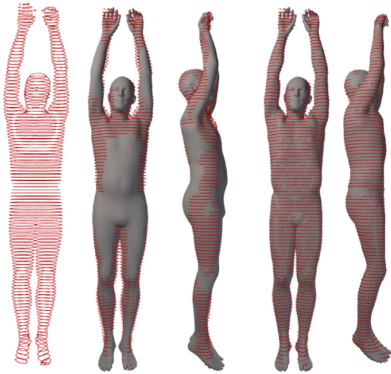
Figure 5. Initial fit to the MRI skin point-cloud. Left: point-cloud S_i extracted from the MRI. Middle: SMPL model fit S_i^1 . Right: Free-vertex fit F_i^1 .
