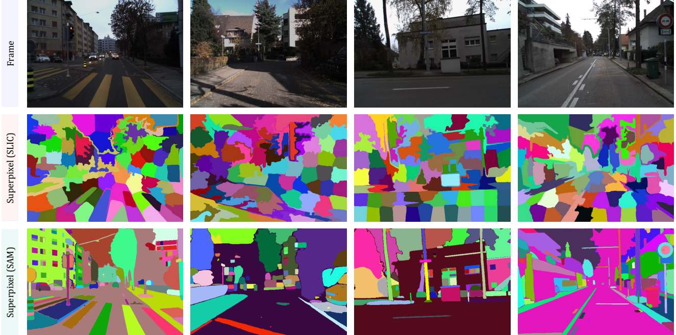
Figure A. Examples of superpixels generated by SLIC [1] (the 2nd row) and SAM [10] (the 3rd row). The parameter M_{slic} in the SLIC algorithm is set to 100. Each colored patch represents one distinct and semantically coherent superpixel. Best viewed in colors.
