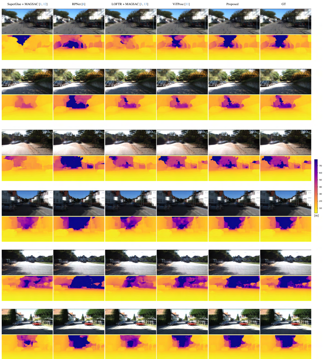
Figure 4. KITTI [7] Qualitative Assessment. We overlay here the rectified left-right stereo pairs. Each column represents a different rectification method. To visually evaluate the rectification quality, focus on an object in the scene and compare the vertical disparity. Every row is accompanied by the corresponding depth inferred from HITNet [14].
