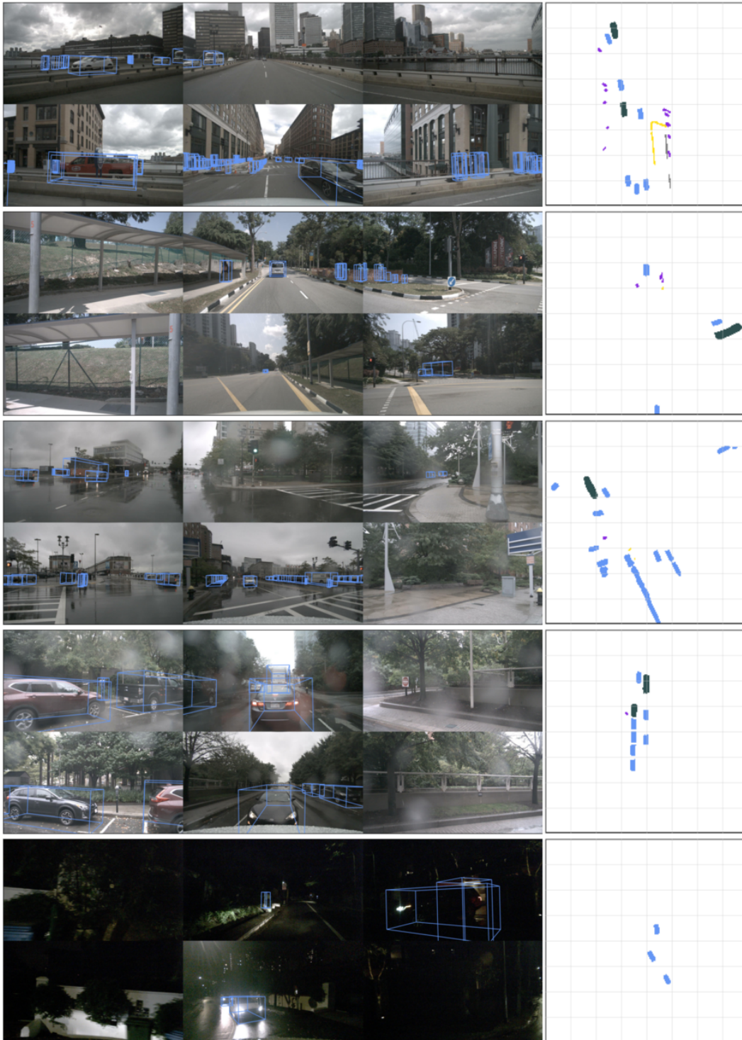
Figure 9. nuScenes Qualitative Results. The first row shows the front_left, front, and front_right cameras, while the second row shows the back_left, back, and back_right cameras. [Key: Cars, Vehicles, Pedestrian, Cones and Barrier of BEVerse-S+SeaBird at 200 \times 200 resolution in BEV ].
