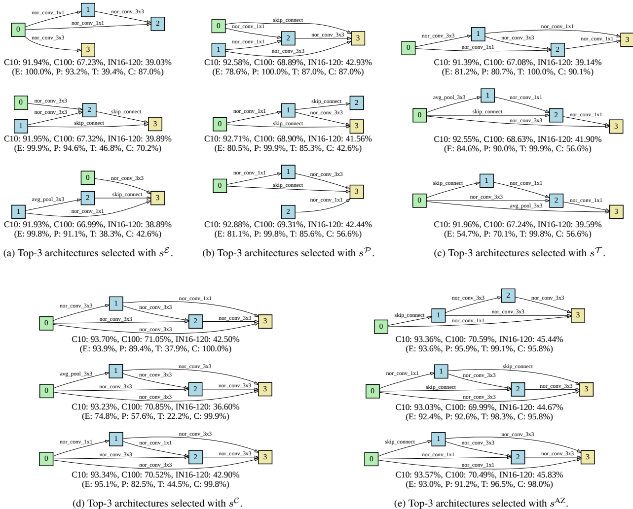
Figure F. Visualization of the top-3 network architectures found with each zero-cost proxy score of AZ-NAS and the final AZ-NAS score on NAS-Bench-201 [7]. The green and yellow squares indicate the input and output nodes of a cell, respectively, and the blue ones represent intermediate nodes. For each architecture, we report the top-1 test accuracies on the CIFAR-10/100 (C10/C100) and ImageNet16-120 (IN16-120) datasets, together with the percentiles for the proxy scores in parenthesis, where 100% indicates the highest ranking. We denote by E, P, T, and C the expressivity, progressivity, trainability, and complexity proxies, respectively, for brevity.
