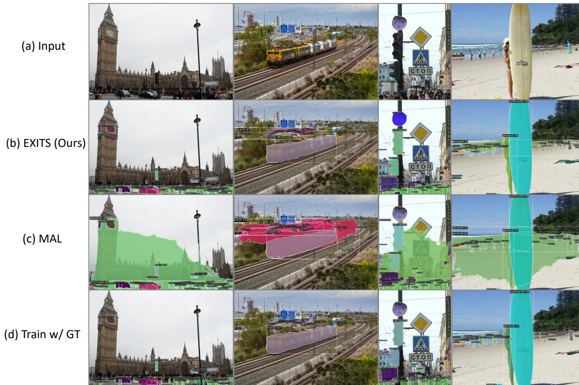
Figure a3. Qualitative comparison of instance segmentation results in complex scenes. (a) inputs (b) EXITS (ours), (c) model train with pseudo labels from MAL [10], (d) model train with the ground-truth label.
