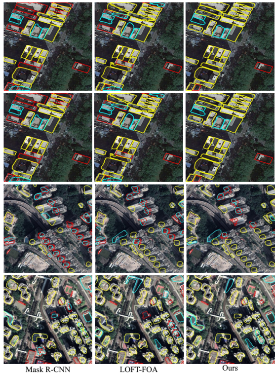
Figure 6. The footprint segmentation results of different models trained on OC_{100} and BH_{100} , respectively. The first two rows display the results of New York (OmniCity-view3), and the last two rows display the results of Hong Kong (HK dataset).
