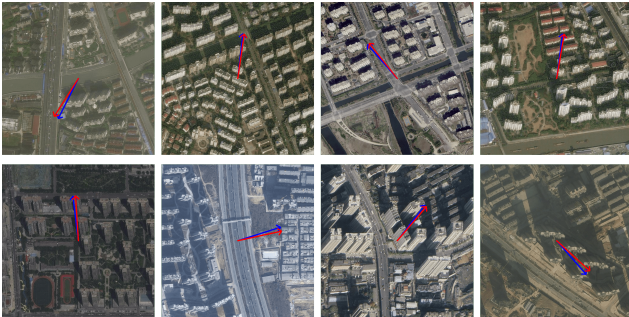
Figure 8. The offset angle prediction results of Shanghai (the first row) and Xi'an (the second row). The red line with the arrow denotes the offset angle ground truth, while the blue line with the arrow denotes the predicted offset angle.
