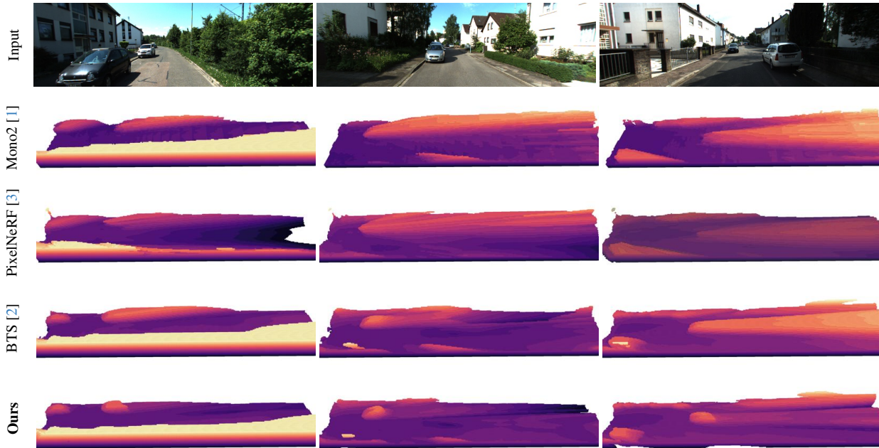
Figure 3. Qualitative comparisons on KITTI-360 dataset (part-1). The scene reconstructions are represented as occupancy grids, where the camera is on the left side and points to the right along the z -axis.
