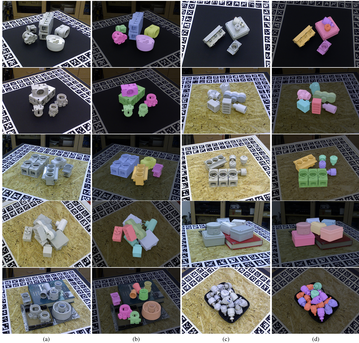
Figure 1. Qualitative results on T-LESS [8]: (a, c) The original images and (b, d) MRC-Net object pose predictions. The object's 3D model is projected with estimated 6D pose and overlaid on original images with distinct colors. Mask RCNN [7, 10] detection is used. Best viewed when zoomed in.
