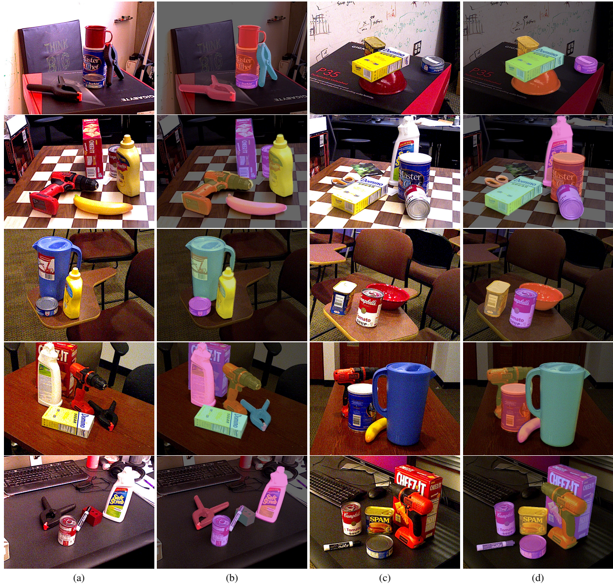
Figure 2. Qualitative results on YCB-V [22]: (a, c) The original images and (b, d) MRC-Net object pose predictions. Mask RCNN [7, 10] detection is used. Best viewed when zoomed in.
