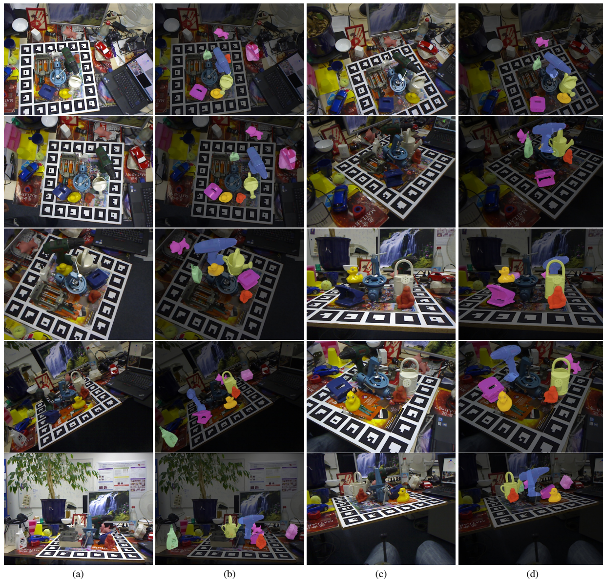
Figure 3. Qualitative results on LM-O [1] : (a, c) The original images and (b, d) MRC-Net object pose predictions. Mask RCNN detection [7, 10] is used. Best viewed when zoomed in.
