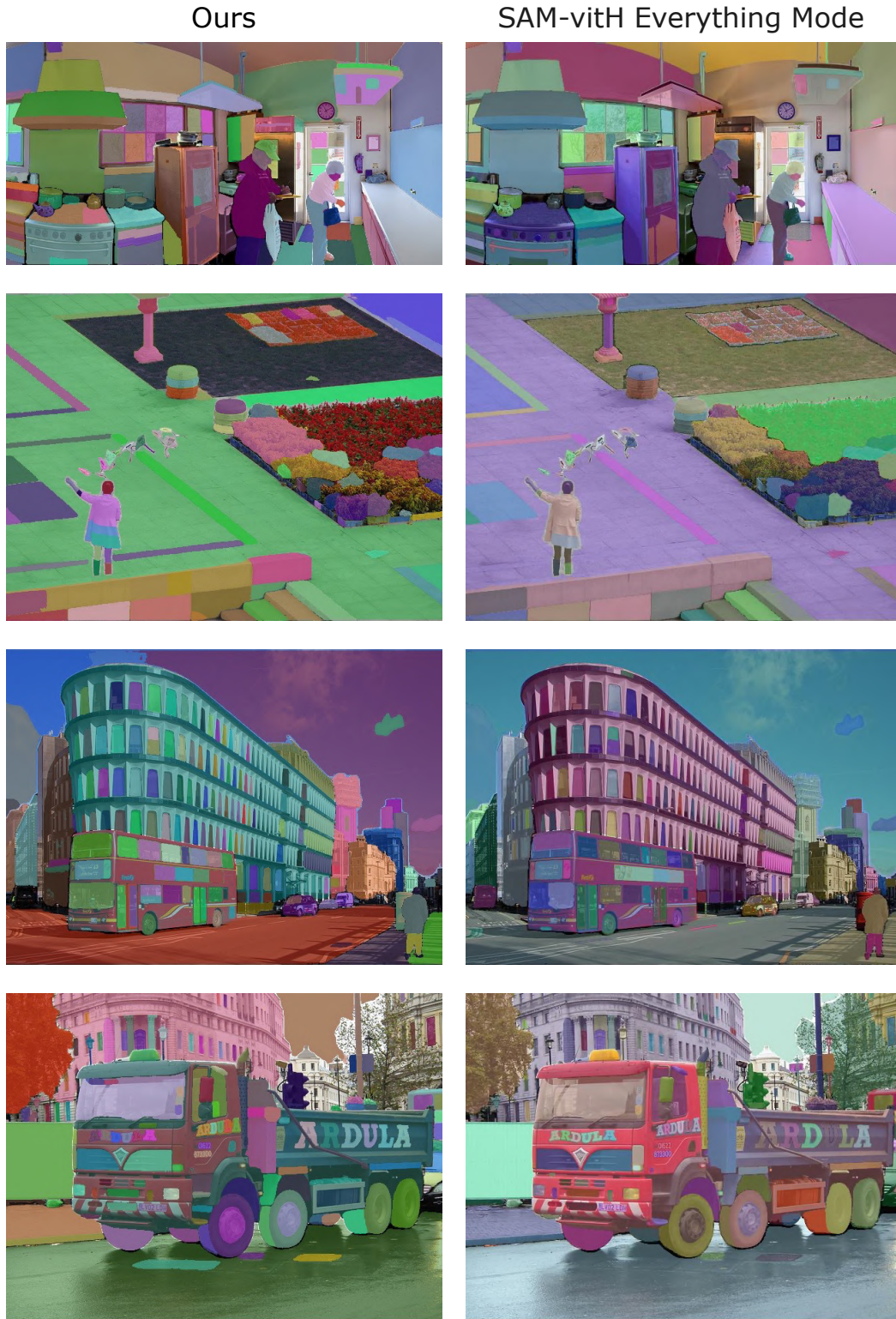
Figure 9. Qualitative comparison between our fast proposal generation and the original SAM everything mode on images from COCO validation set. The results show that our fast proposal generation can achieve similar segmentation quality to the everything mode of SAM, despite using much less time.
