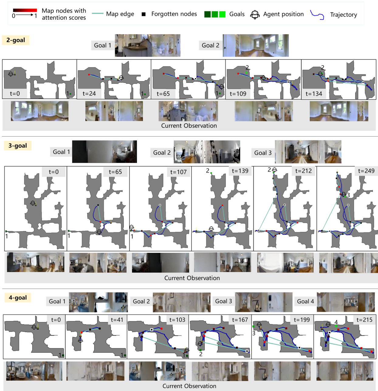
Figure 12. Multi-goal example trajectories of MemoNav. Each example shows both the topological map and the trajectory. The graph nodes are incrementally added to the map and selectively retained by the forgetting module in MemoNav. The examples illustrate that MemoNav flexibly neglects distant nodes. The yellow downward arrow denotes the current localized node of the agent. The comparison with VGM in these example tasks is recorded in the supplementary videos.
