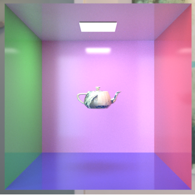
Figure 3. Scene setup of the synthetic dataset. We placed the object inside a modified Cornell Box. The light bounces multiple times and becomes polarized before hitting the object.
