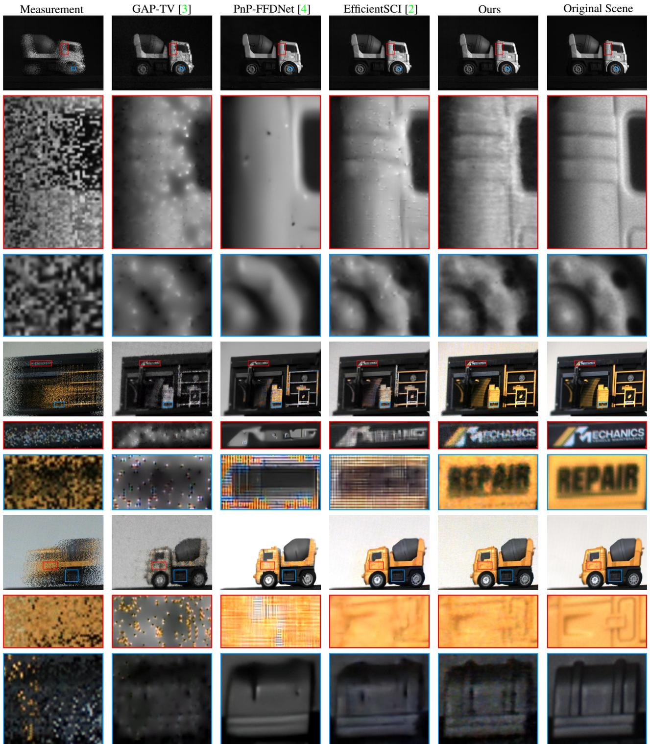
Figure 3. **Qualitative evaluations of our method against SOTA SCI image restoration methods with real dataset.** Top to bottom shows different scenes. Since compressed ground truth images are unavailable, we captured separate scene images after capturing SCI measurement. The qualitative comparisons demonstrate that our SCINeRF surpasses prior methods on image reconstruction with real dataset.
