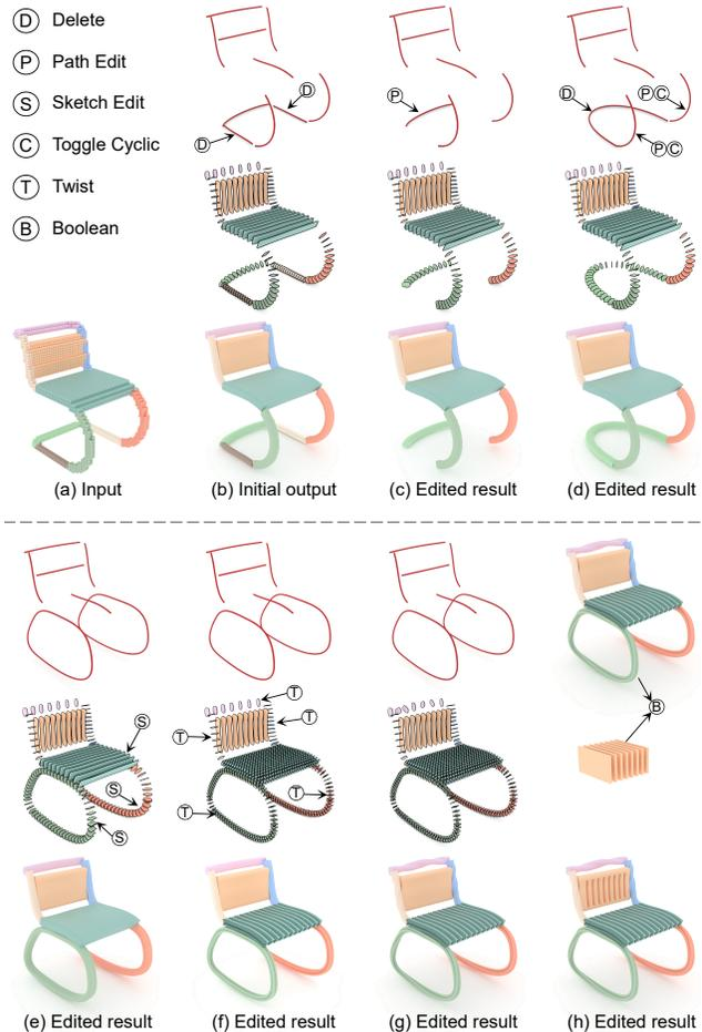
Figure 1. Varieties of methods for editing and further creating based on the output of SfmCAD. Columns (b-g) sequentially present the shape’s path, sketch, and a representation of sketch+path, from top to bottom.
