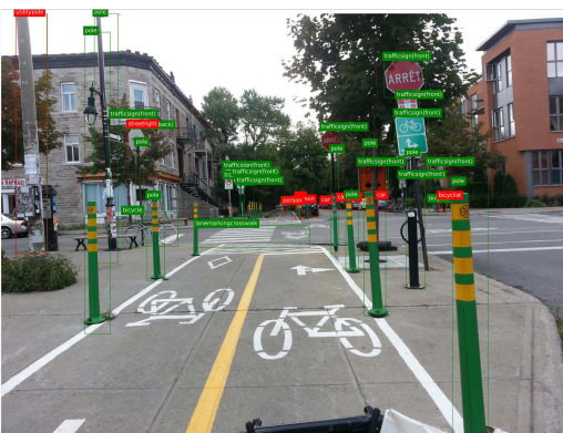
Figure 4. Visualization of the detection results under different methods. We treat a box prediction as true positive if it has an IoU larger than 0.5 with the ground-truth box. The true positive predictions are in green color, while the false positive predictions are in red color. Top-left: Semi-supervised Learning (Semi-SL) method, i.e., Unbiased Teacher-v1 [2]. Top-right: Open-vocabulary object detection (OVOD) method, i.e., OWL-v2 [4]. Bottom-left: AIDE. Bottom-right: ground-truth.
