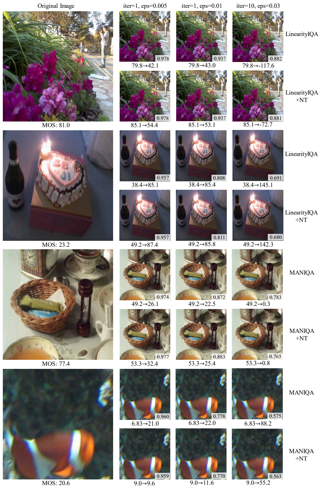
Figure S7. (Zoom in for a better view) Visualization results of adversarial examples generated using the FGSM with different intensities. The normalized MOS is presented. FGSM attack settings are indicated above the figures, and each adversarial example for a model is presented with the format: “predicted score before attack → predicted score after attack” below the respective images. The SSIM between the adversarial example and the original image is displayed at the bottom right corner of each adversarial image.
