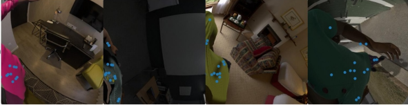
Figure 2. Self-occlusion visualization; blue dots are keypoints. human-object interactions that are not possible to mimic without simulating the objects (such as sitting on chairs). Since each capture session contains a long sequence of motion, we further divide the sessions into sequences that contain around \sim 450 frames of motion, resulting in a total of 5169 sequences for training and testing.
