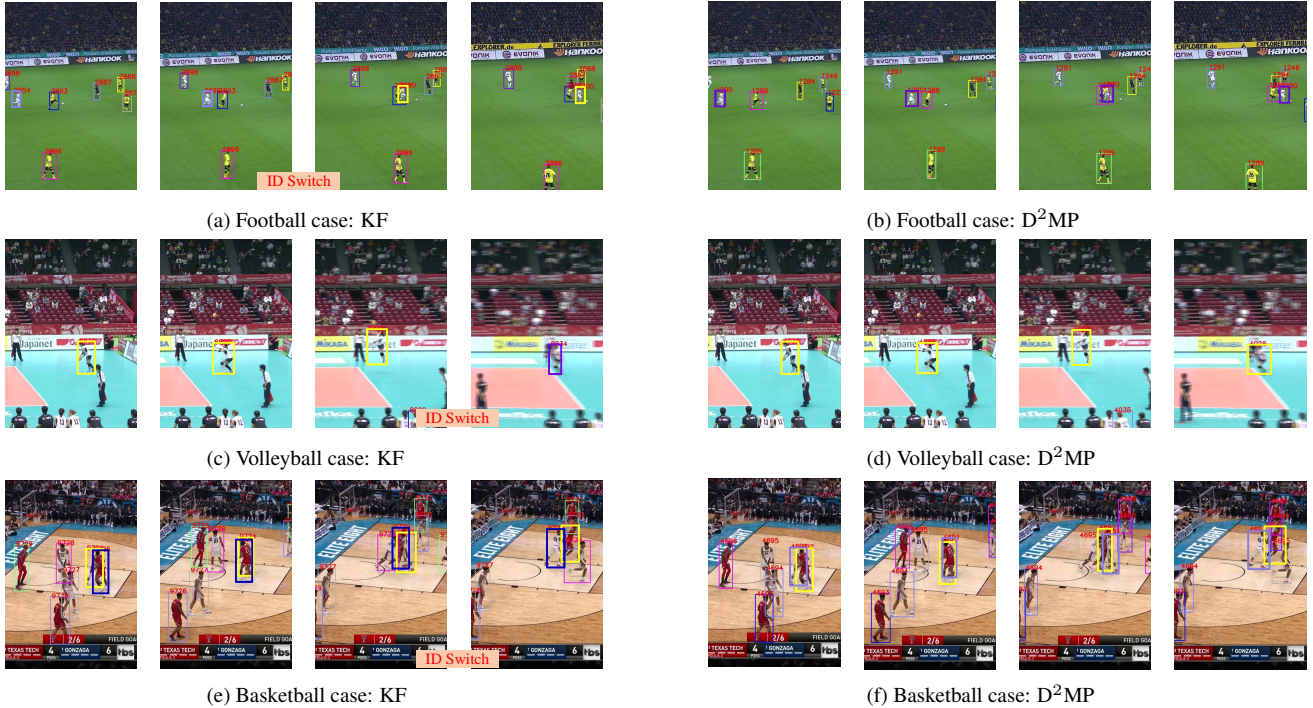
Figure 3. Qualitative comparison between using KF or D^2MP as the motion model on the SportsMOT test set. (a), (c), and (e) represent the results using KF as the motion model. (b), (d), and (f) represent the results using D^2MP as the motion model. Each pair of rows shows the comparison of the results for one sequence. All of the cases are in scenarios with a moving camera. Boxes of the same color represent the same ID. Best viewed in color and zoom-in.
