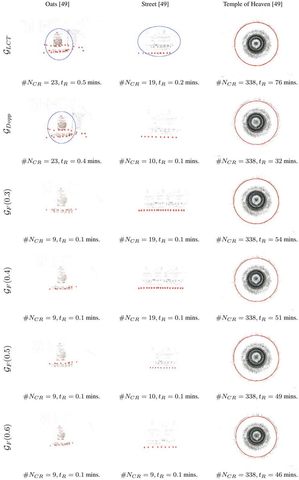
Figure S10. Reconstructions obtained with different graphs on ambiguous datasets from [49] where superimposed parts of the reconstructions are marked in blue. \#N_{CR} : Number of cameras reconstructed, t_R : Reconstruction time using COLMAP [36]. Recommended minimum edge score ( m ) for small-scale datasets: 0.3 to 0.4.
