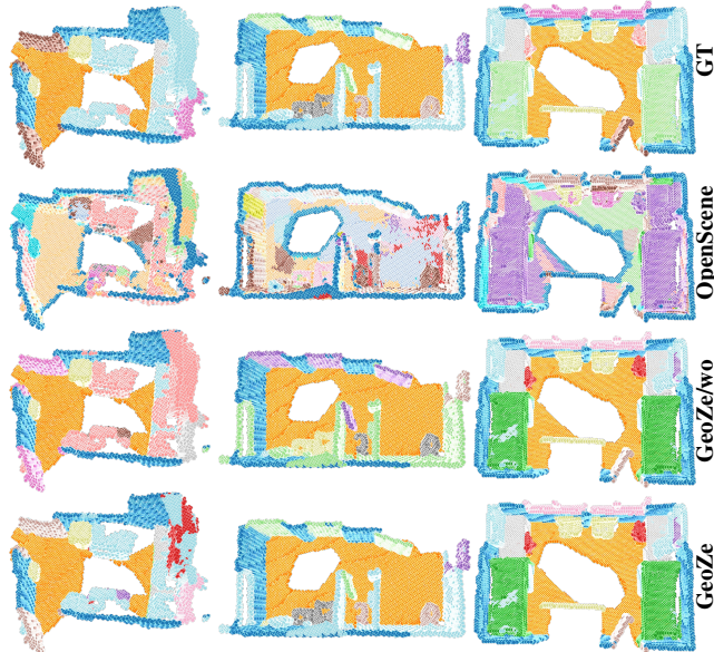
Figure 1. Zero-shot semantic segmentation results on ScanNet using OpenSeg feature extraction. (top row) ground-truth annotations, (second row) OpenScene (OpenSeg) [6], (third row) GeoZe/wo (OpenSeg) without using VLM representation anchors, and (bottom row) GeoZe (OpenSeg). ‘wo’ indicates the absence of VLM representation anchors.
