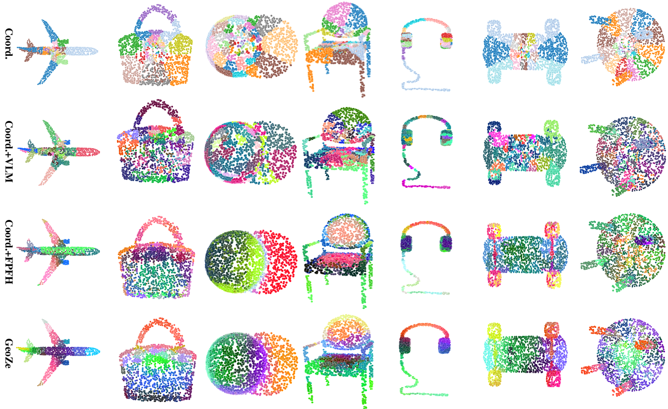
Figure 5. Visualization of clustering results on ShapeNetPart [11] using various sources: (top row) coordinates only; (second row) coordinates with VLM representations; (third row) coordinates and geometric representations (FPFH); (fourth row) coordinates and geometric representations (FPFH), guided by VLM representation similarity. Coord. represents Coordinates.
