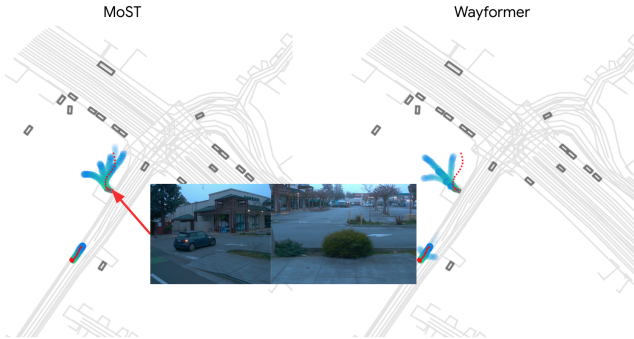
Figure 1. Additional qualitative comparison between MoST and Wayformer [3] baseline. The agent boxes are colored by their types: gray for vehicle, red for pedestrian, and cyan for cyclist. The predicted trajectories are ordered temporally from green (+0s) to blue (+8.0s). For each modeled agent, the models predict 6 trajectory candidates, whose confidence scores are illustrated by transparency: the more confident, the more visible. Ground truth trajectory is shown as red dots. Note that the vehicle indicated by the red arrow is entering a plaza which has no map coverage. Since our model has access to the rich visual signals, it correctly predicts the vehicle’s possible trajectory which includes follows the arrow and turn right. Wayformer, on the other hand, completely missed this possibility due to the lack of road graph information in that region.
