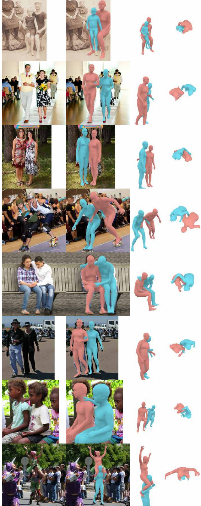
Figure 1. Flickr Fits. We visualize the output of the optimization process that reconstructs two people in close proximity using ground-truth contact maps, shown from three different views.
