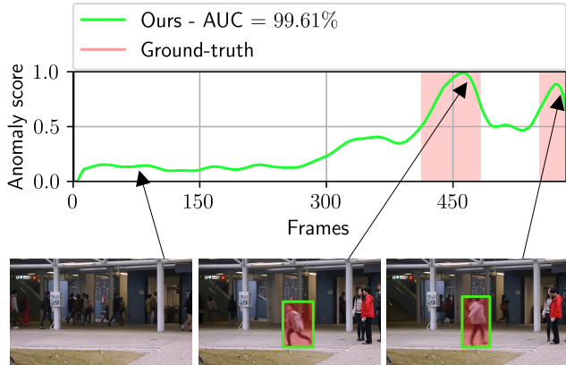
Figure 3. Predictions for test video 07 from Avenue. The abnormal bounding boxes are given by the convex hull of the patches labeled as abnormal. Best viewed in color.
