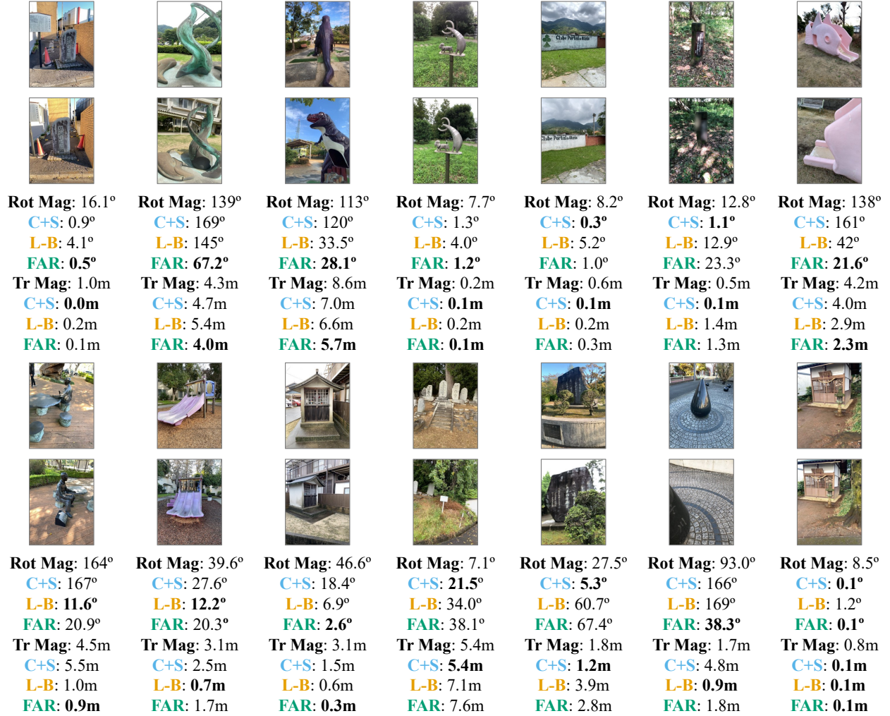
Figure 6. Random results on Map-free Relocalization. C+S: LoFTR + Solver. L-B: 6D Reg [1]. FAR: uses 6D Reg features and LoFTR correspondences. FAR is often best, having minimum rotation error 7 instances vs. 5 for C+S and 2 for L-B, and minimum translation error 7 times vs. 7 for C+S and 3 for L-B. C-S has far worse errors in failure cases than FAR (e.g. row 1 column 7).
