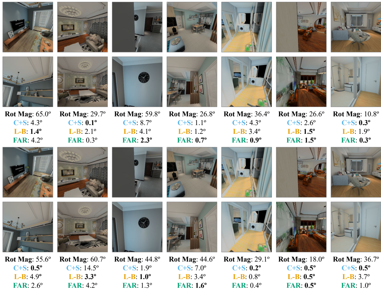
Figure 7. Random results on InteriorNet. C+S: LoFTR + Solver. L-B: 8-Point ViT. FAR: uses 8-Point ViT features and LoFTR correspondences. FAR has the lowest error more frequently than alternatives, and has the lowest maximum error: 4.2° vs. 4.9° for L-B and 14.5° for C-S.
