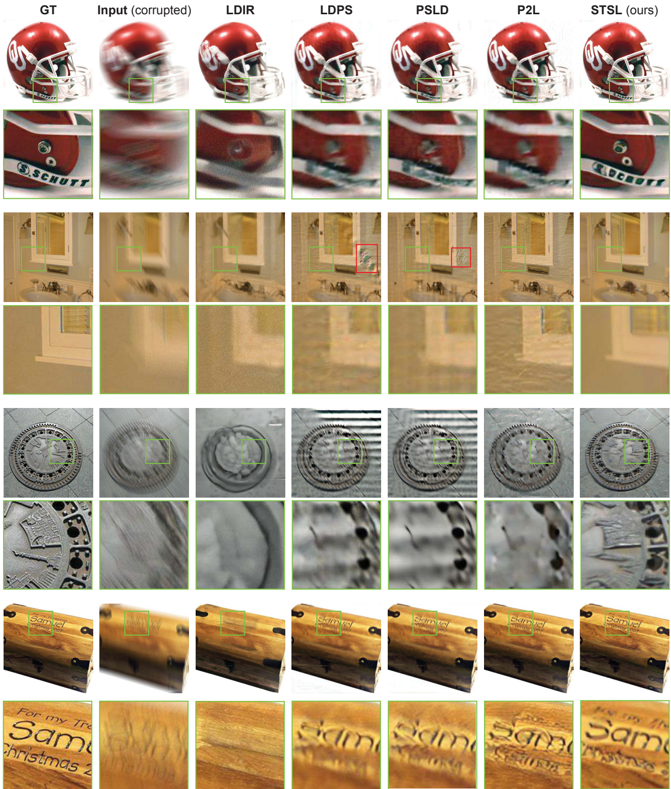
Figure 4. Qualitative results on motion deblurring: Odd rows represent the full image, while even rows show a zoomed-in view of the green box . The red boxes indicate artifacts from various methods. STSL demonstrates superior performance in preserving image details while simultaneously minimizing artifacts and fake textures. The competitive baselines: PSLD [43] and P2L[10] introduce artifacts and fake texture that might be mistaken as sharpness of the reconstructed image. Observe the high fidelity text restoration by the proposed approach STSL in the last row.
