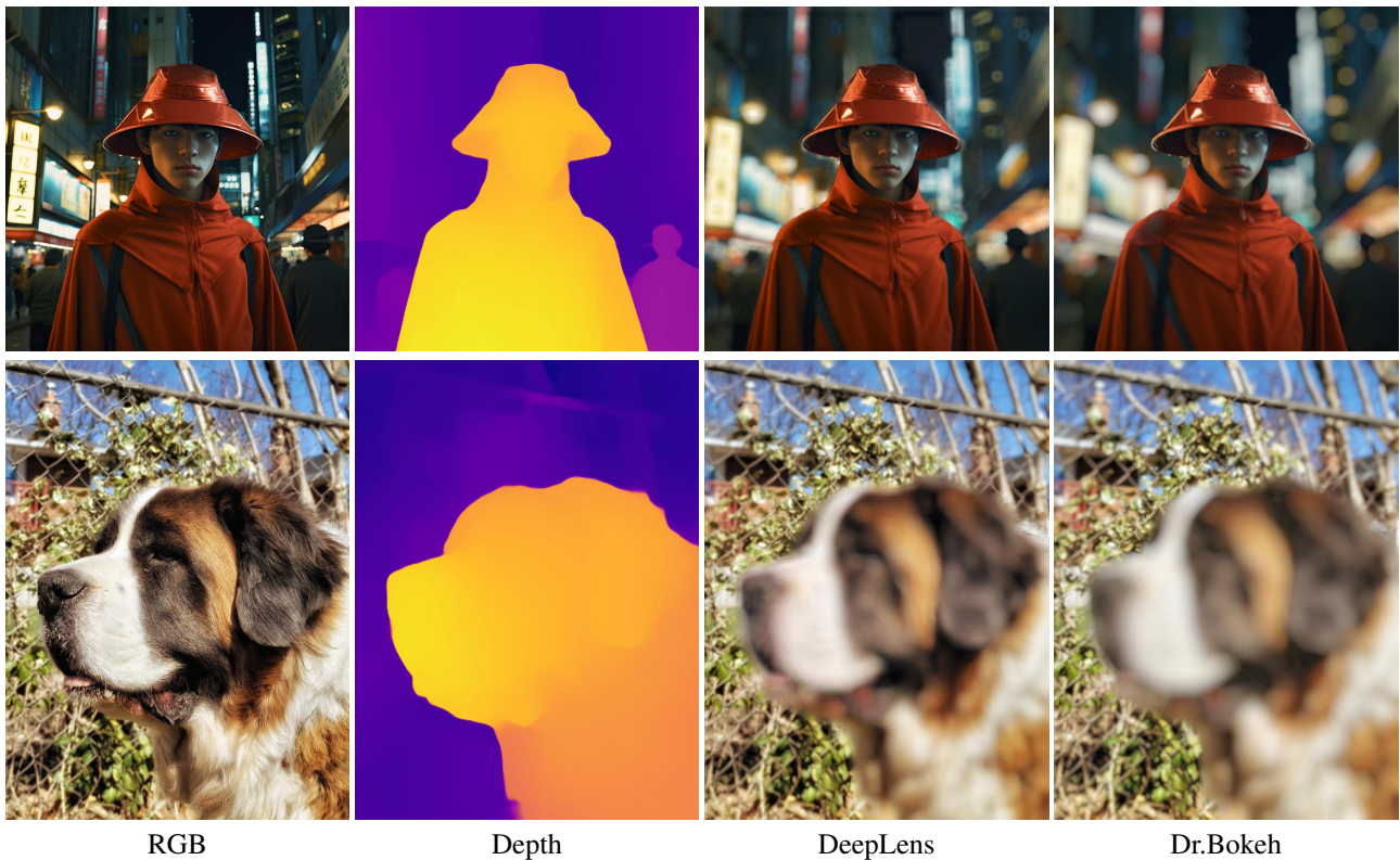
Figure 4. DeepLens problem: 1. The bokeh shape is not well preserved by DeepLens; 2. The boundary soft transition is not smooth in the partial occlusion boundary. Best viewed by zoom-in.
