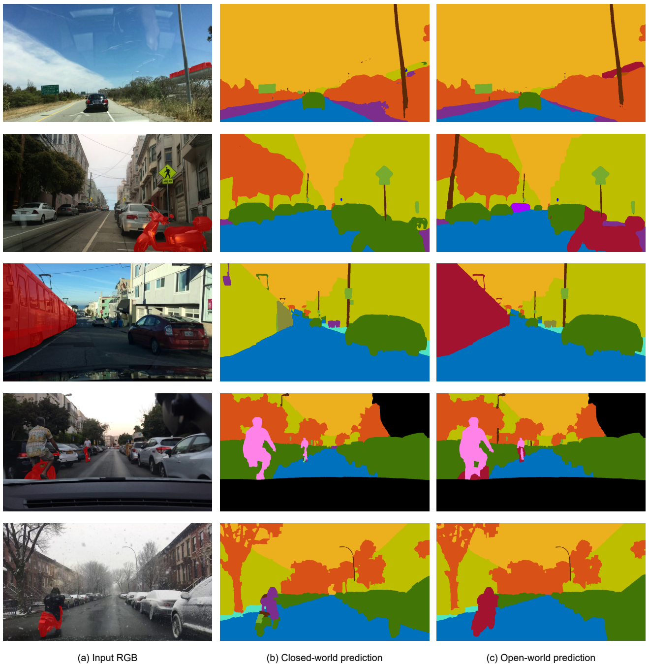
Figure 6. Anomaly segmentation results from the test set of BDDAnomaly. We show the input RGB overlaid with the ground truth unknown mask (a), the prediction of our closed-world model (b), and the prediction of our approach for open-world segmentation (c). In the open-world prediction, the unknown class is shown in red. Notice how the two models, that are both trained on BDDAnomaly, perform similarly on known classes, demonstrating that our approach does not degrade closed-world performance.
