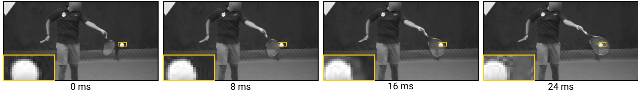
Supplementary Figure 19. Sequence used for UltraPhase experiments. This sequence covers 2500 binary frames (25.8 ms). The cropped portion captures the edge of a swinging racket as it makes contact with a tennis ball.
