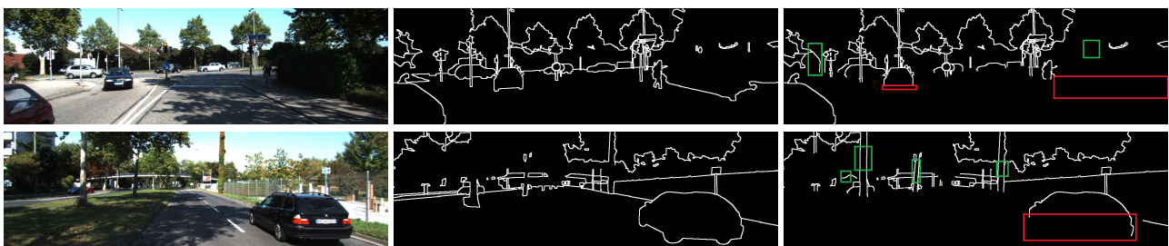
Figure 13. Examples of the annotation process (the edges are dilated for visualization purposes). (a) The RGB image. (b) The edges of the instance segmentation GT. (c) The depth edges GT, where green and red rectangles exemplifies edge addition and deletion, respectively.
