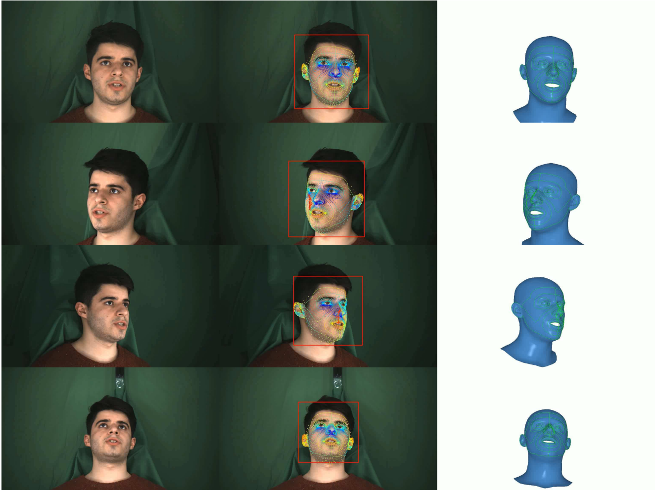
Figure 21. 3D data generation using the MEAD [40] dataset. Our face tracker can seamlessly integrate multiple-view video to improve 3D face tracking. Extrinsic, intrinsic and the 3D face model (right column) are simultaneously optimized to fit the predicted 2D alignment (center column) in our 3D model fitting module. We utilize 4 cameras for each sequence to generate high quality training data for speech-driven 3D face animation models.
