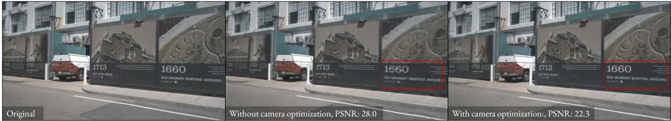
Figure 10. Effect of camera optimization on nuScenes. Despite clearly sharper image quality, we get drastically reduced PSNR scores when using camera optimization. This is due to the misalignment between the learned poses and the evaluation poses. This can be seen in the far left of the image, where the image with camera optimization displays less of a window.
