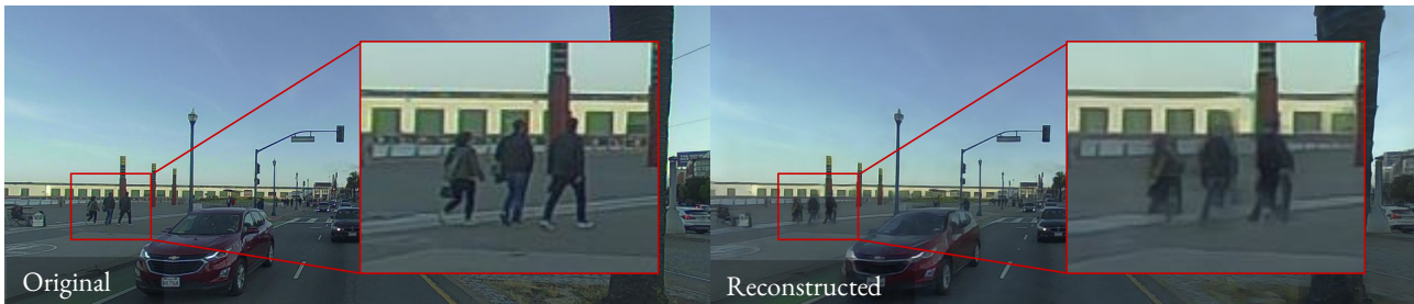
Figure 11. Failed reconstruction of deformable actors. The assumption that all actors are rigid is invalid for pedestrians and the like, leading to blurry reconstruction as seen here.
