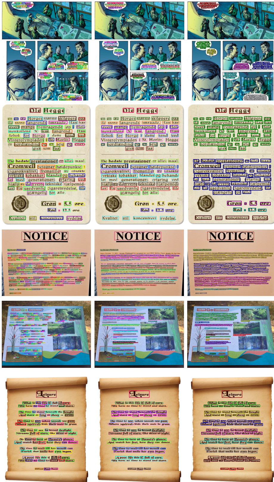
Figure 5. Visualization results of hierarchical text detection. Columns 1-3 represent the detection results for word, line, and paragraph levels, respectively. Text instances belonging to the same hierarchical level are enclosed within rectangles of the same color. (The figure is best viewed in color.)
