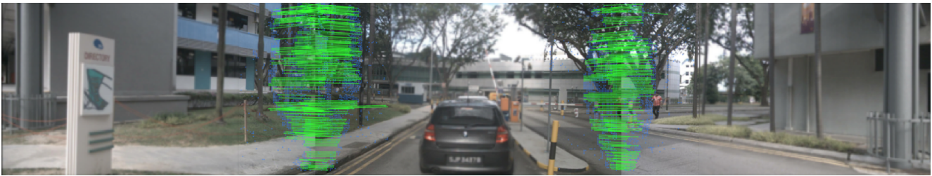
Figure 22. Illustration of keypoint matching in KPM calculation. The blue points are the image keypoints in the overlapping regions on the left/right side of the image. The green lines are the matched keypoints between the current view and its two adjacent views using the LoFTR [56] matching algorithm.
