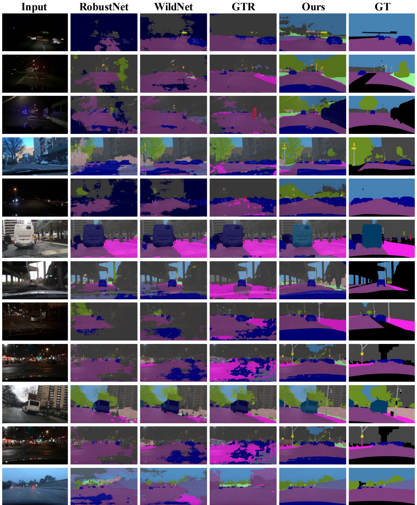
Figure 2. Prediction results of DINOv2+Rein on the BDD100K validation set. The model is fine-tuned exclusively on the GTAV dataset, without access to any real-world urban-scene datasets.
