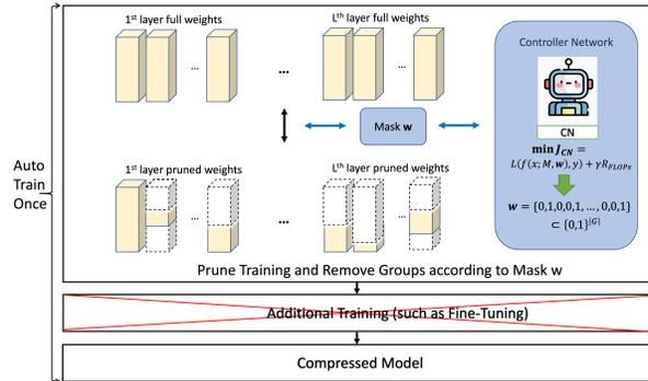
Figure 1. Overview of Auto-Train-Once (ATO). The controller network generates mask  $w$  based on the size of ZIGs  $\mathcal{G}$  to guide the automatic network pruning of the target model and we remove variable groups according to mask  $w$  after training. Additional training (such as fine-tuning) is not required after model training and we can directly get the final compressed model.
