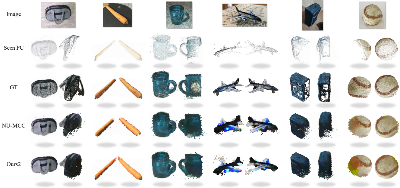
Figure S1. More qualitative comparison of reconstructions by Ours2 and NU-MCC, evaluated on CO3D-v2 held-out categories. We visualize two views for each seen, GT, and predicted point cloud by NU-MCC and Ours2.
