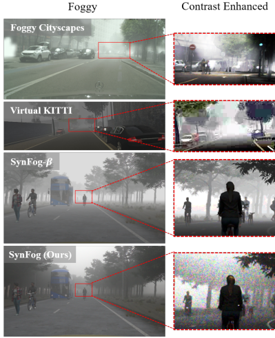
Figure 4. Comparison of SynFog with other synthetic datasets in the driving field. The second column displays the result after regional contrast stretching of the rectangular region, revealing that only SynFog exhibits consistent noise characteristics with those found in real captured foggy images.
