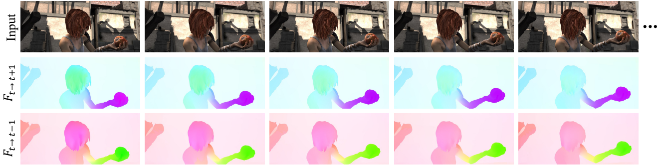
Figure 11. Optical flow labels for Sintel [1] dataset. The first row is video frames of Sintel dataset, and the second row is ground-truth forward optical flow from frame t to t+1 . The Sintel does not provide backward flow. Therefore, we use pre-trained RAFT [34] flow network to generate backward optical flow from frame t to t-1 as pseudo-labels, shown in the third row.
