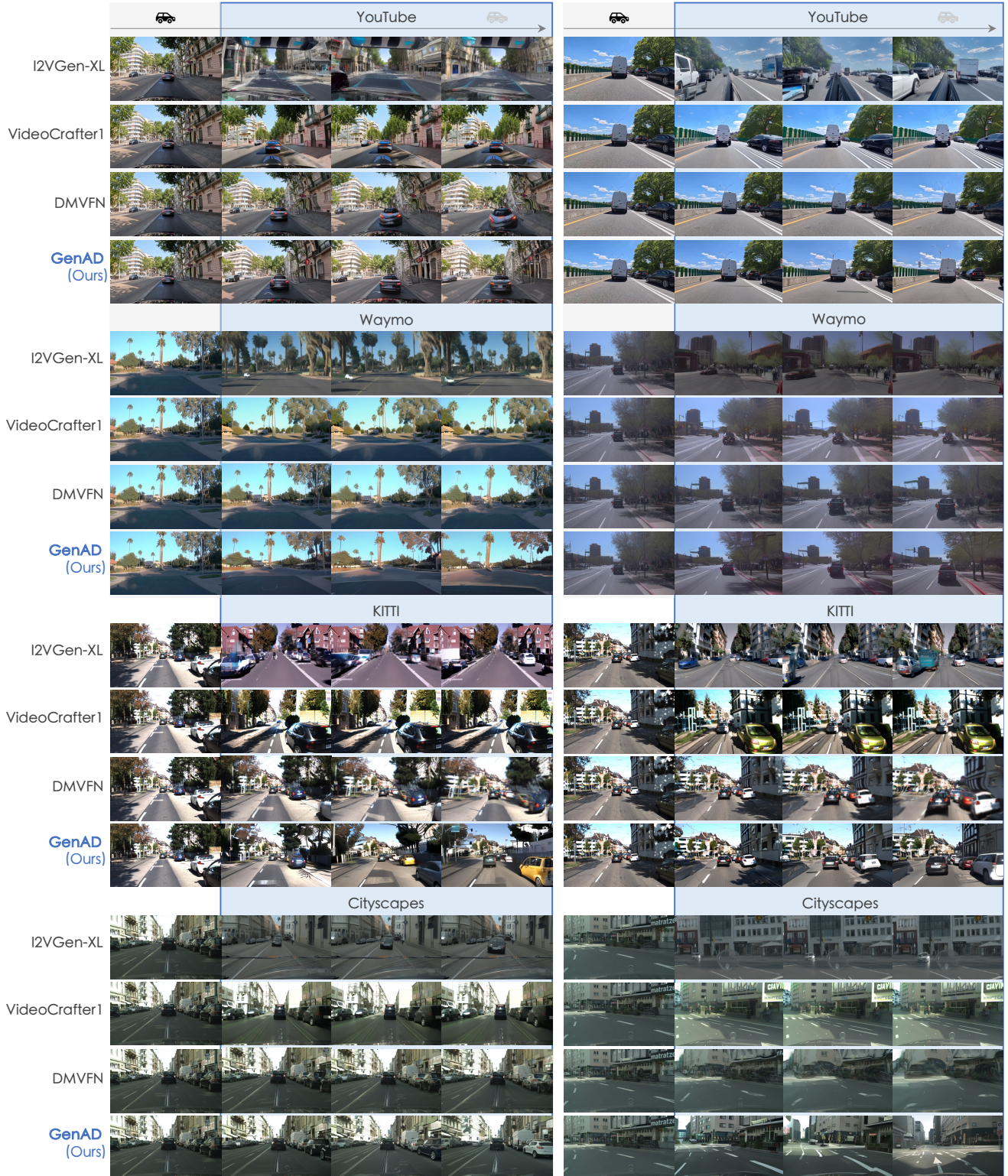
Figure 7. Zero-shot video prediction on public datasets compared with state-of-the-art video generation/prediction models. Videos generated by I2VGen-XL are inconsistent with the condition frame. VideoCrafter1 appears to generate static scenarios. DMVFN suffers from huge image distortions. Meanwhile, all the other 3 models fail to generate videos when the ego vehicle should turn to the left and follow the lane (see the rightmost case in the last row). Our model manages to succeed in predictive video generation with great consistency with the conditional frames. We only show the first, third, and fifth frames from 6 predicted frames of our model due to space limits.
