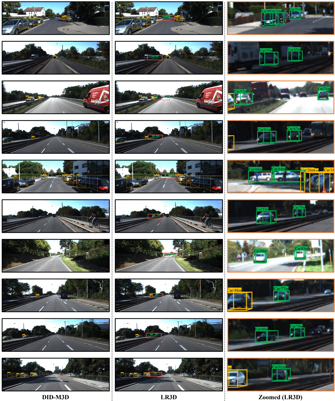
Figure 3. Qualitative comparison results between DID-M3D [12] with (middle, LR3D ) and without (left, DID-M3D ) LR3D long-range teacher on detecting distant objects beyond 3D bounding box label range. The newly detected distant objects with their predicted 3D bounding boxes are marked in green . As illustrated, though only trained with limited range of available 3D annotations within 40m, LR3D enables DID-M3D to accurately detect distant objects beyond this range.
