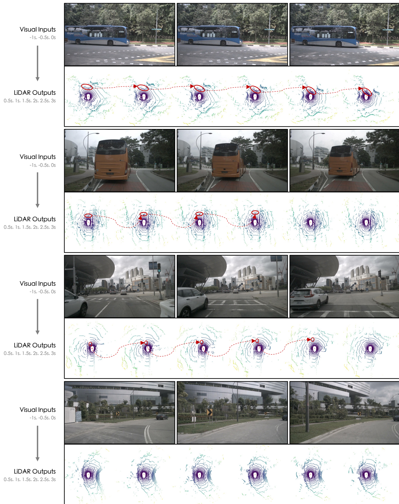
Figure 4. Qualitative results of ViDAR for visual point cloud forecasting on nuScenes validation set. Top: historical visual inputs in 1 second; bottom: future point cloud predictions in 3 seconds. The first, second, and third rows provide examples of modeling relative motions between the ego-vehicle and other parked or moving objects (highlighted in red circles ); the fourth row shows the future estimation where the ego-vehicle is turning right. As illustrated, ViDAR effectively captures the information of 3D geometry and temporal dynamics, and thus correctly estimates future point clouds from visual sequence inputs. All point cloud visualizations are under the ego coordinates.
